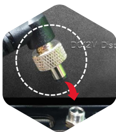
Tighten connection for power
