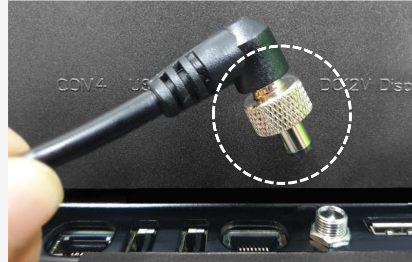
Power Supply Secure Fastening Structure
