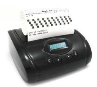
CompArt International introduces new VLINE-112 thermal printer. Due to innovative, compact design, battery power supply and various interface types, VLINE-112 printer is dedicated for both stationary and mobile use.
