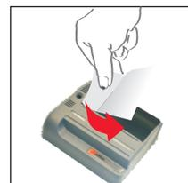
Grab the printout protruding from the printer with your hand. Pull it vigorously and diagonally to the direction of its ejection in such a way that the printout is lying against the cutter bar contained in the printer housing.
