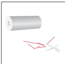
Before the paper is inserted into the printer, one should clip its end..
