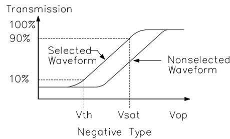
**Vth:** The voltage Vop which the transmission rate of segment is 90%(positive) or 10%(negative) of saturated value on conditions of the selected waveform.(non-selected waveform is opposition)
